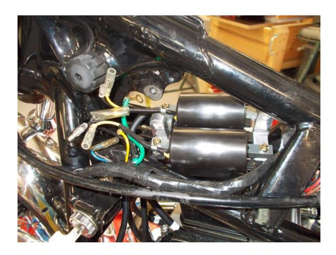
9. Be sure to clean the paint from the frame where the front coil bracket attaches to the frame, some models use this for a grounding point.
