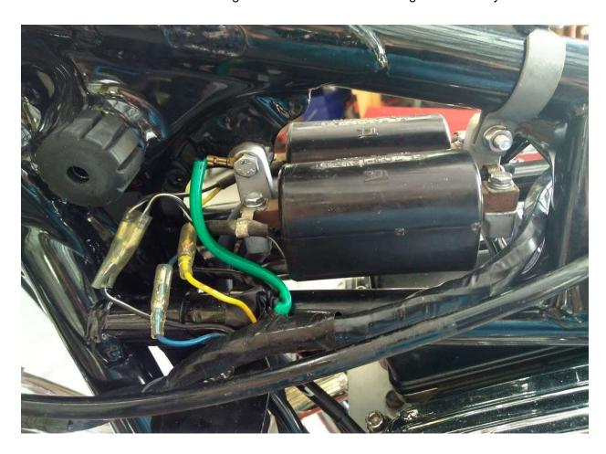
7. Begin installation of the new coil assembly. Start from the right side being careful to feed the spark plug wires down through the frame rails in the direction of the spark plugs.
